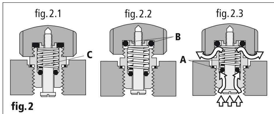
During the decompression phase, unscrew the crown of the valve in order to release the mechanism (fig. 2.2). The valve is now watertight from the outside. As the interior pressure becomes greater than the exterior pressure, it pushes the gasket (A) out of its seating, thus releasing the gas (fig. 2.3). Once the pressure is equalised, gasket (A) returns to its original position, pushed by the spring (C) (fig. 2.2).
