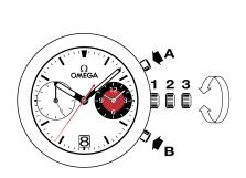
Timing to 1/8 of a second for up to 12 hours.
