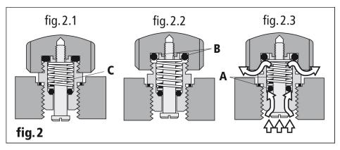
During the decompression phase, unscrew the crown of the valve in order to release the mechanism (fig. 2.2). The valve is now watertight from the outside. As the interior pressure becomes greater than the exterior pressure, it pushes the gasket (A) out of its seating, thus releasing the gas (fig. 2.3). Once the pressure is equalised, gasket (A) returns to its original position, pushed by the spring (C) (fig. 2.2).
