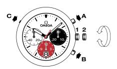
Timing to 1/8 of a second for up to 12 hours.
